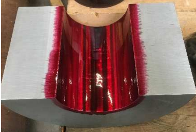
Verification of the absence of cracks by dye penetrant testing
